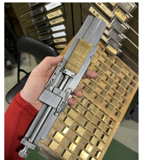
The composing stick and jobcase for the Ludlow.
